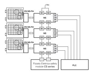
Possible connection in series of several switches in order to simplify the safety system wiring, after evaluating the outputs from the last switch in the chain by means of a Pizzato Elettrica safety module (table for safety modules to be combined). Each NS series switch is provided with two signalling outputs which are activated when the guard is closed (O3) or locked (O4). This piece of information can be managed by a PLC, depending on the specific requirements of the system installed.
