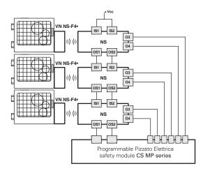
Possible connection in series of several switches in order to simplify the safety system wiring, after evaluating the outputs from the last switch in the chain by means of a safety module from Pizzato Elettrica CS MP series, which allows management of both safety and signalling functions.
