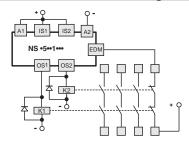
The NS •5••1••• version, in addition to maintaining the operating and safety characteristics of the NS series, allows control of **forcibly guided NC contacts of contactors or relays** controlled by the safety outputs of the switch itself. As an alternative to the relays or contactors you can use Pizzato Elettrica expansion modules CS ME-03. See page 235 - CATALOGUE SAFETY 2015/16. This check is carried out via the EDM input (External Device Monitoring as defined in EN 61496-1) of the switch.
