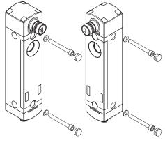
operation such as rotating the module where the actuator is to be inserted. The fixing holes can then be sealed with the protection caps supplied, in order to avoid any possible accumulation of dirt and prevent tampering.
