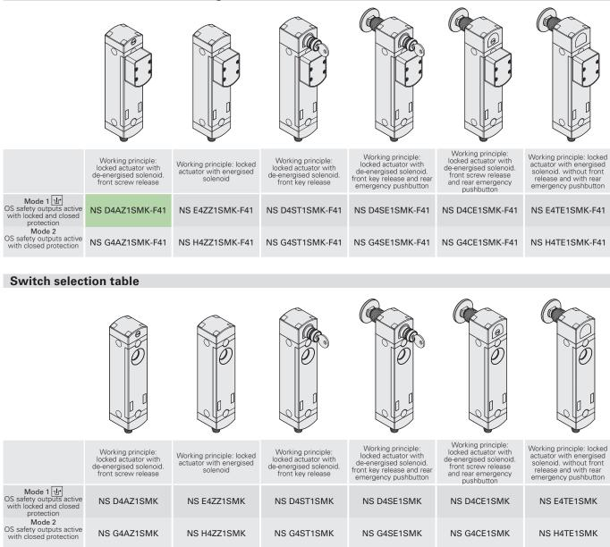
To purchase a product with side connections replace letter S with letter D in the codes shown above. Example: NS D4AZ1SMK → NS D4AZ1DMK To purchase a product with EDM input replace number 4 with number 5 in the codes shown above. Example: NS D4AZ1SMK → NS D5AZ1SMK Legend: <u>u</u> interlock with lock monitoring in accordance with EN ISO 14119
