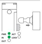
When the actuator leaves the activation limit area, the device turns off the ACT LED and the O3 signalling output.
