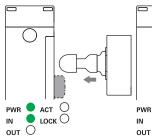
The switch is supplied with power (PWR LED on, green), the IS1 and IS2 inputs are enabled (IN LED on, green), the OS1 and OS2 safety outputs are disabled (OUT LED off). The actuator is on the outside of the activation zone (LED ACT off).
