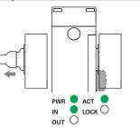
When the actuator is brought inside the safe activation area (dark grey area), the switch turns on the ACT LED (green). In this position, the O3 doorclosed signalling output is activated. The actuator is not locked (LOCK LED off).
